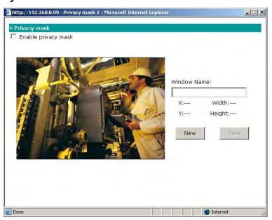
Five private mask areas can be set up for each camera. The areas appear as filled rectangles (with fill color set to black) to hide the privacy of objects in that region. A privacy mask window is set up in the same way as a motion detection window.
